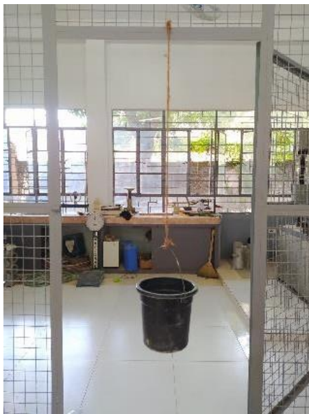
Fig. 12. A BSPF rope carrying a bucket.
