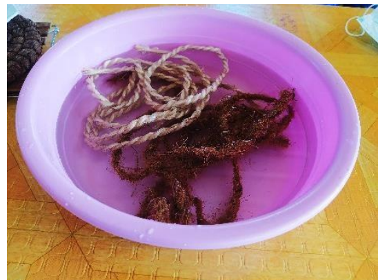
Fig. 10. BPSF ropes and coco fiber ropes soaked in water for 24 hours.
